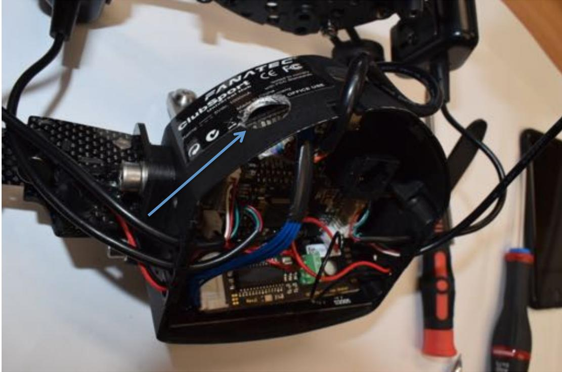
5. Replace the PCB after drilling and flip the board over to reveal the 12 pin connector.
