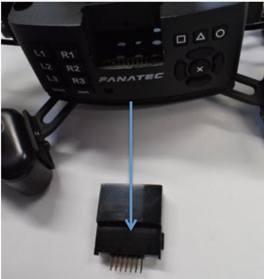
2. Remove the memory data pack and carefully open the hub taking care not to pull on the cables.
